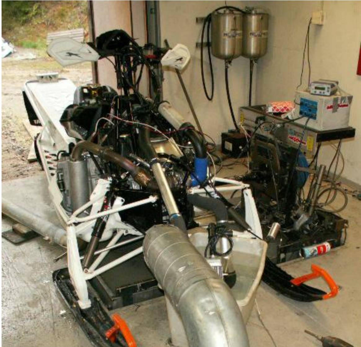
Arctic Cat M1100 turbo during dyno tests in our Superflow engine dyno.
