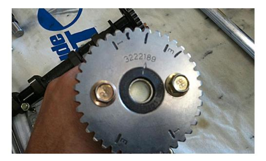
Remove the sprocket from the cam and make the holes a little longer by grinding on one side to elongate the hole (counter-clockwise with the Intake and Exhaust marks facing you). If you grind to holes about 0,6 mm (0,025") wider, the cam settings will be right when turning the cam fully to this direction when installing the cam sprocket bolts.
