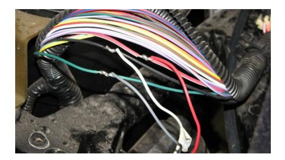
A small MAP (Manifold Air Pressure) signal voltage converter box will need to be installed inline with three of the wires from the stock MAP sensor. This can be done near the MAP sensor or at the bundle where the EFI box wires are connected. The box is labelled with the end that is connected with the ECU end of the wires that are cut as well as the MAP (sensor) end.
