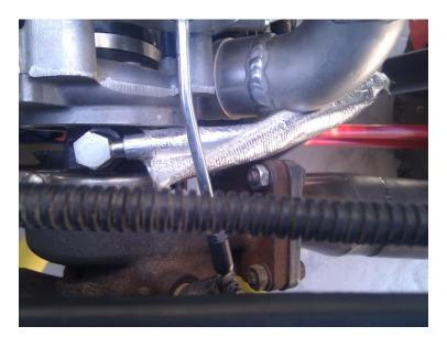
Please be sure that your RZR has the heat shield installed from the factory that goes in front of the header. This is installed on all the newer RZR XPs, but was a retrofit part for the original units. This piece can be purchased from Polaris for a nominal fee if needed.
