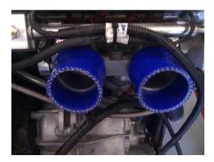
The plenum will be installed on the front of the throttle bodies with the supplied hoses and clamps.
