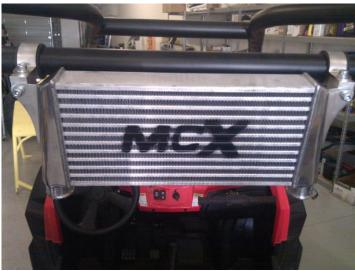
The intercooler will hang from the roll cage with the supplied straps and blocks. The location will be in the middle of the vehicle..
