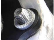
6. A small amount of the passenger side existing muffler bracket will need to be cut off. The supplied muffler mounting hardware will be used to support the muffler as pictured here.
