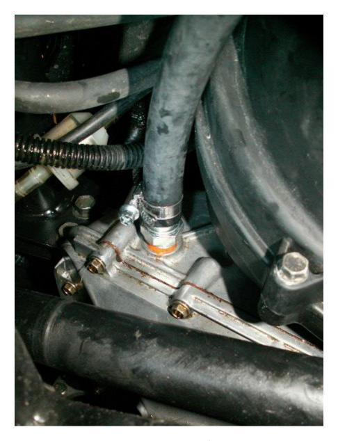
Install the oil return hose between the oil outlet of the turbo and this new oil return fitting on the engine block. Use hose clamps.
