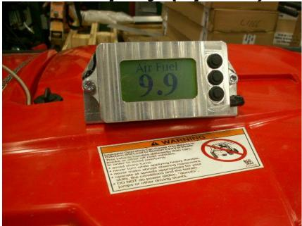
The MCX display can be bought as an option. A wide range oxygen sensor is included. You can watch many different things on the display for instance air/fuel ratio, turbo pressure, rpm, throttle position etc.
