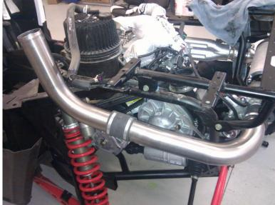
The vent from the oil tank will connect to the intake tube.
