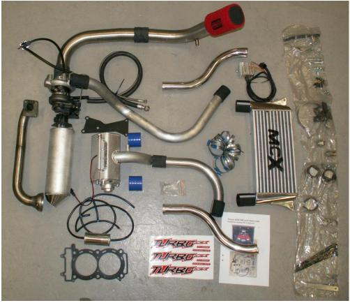
When unpacking the parts, please check inside the tubes, plenum and intercooler for dirt or packing material. Blow with high pressure air, or clean the object if necessary.
