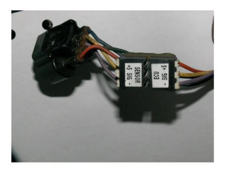
There are multiple yellow and orange wires in the bundle, so it needs to be verified that the correct ones are used.
