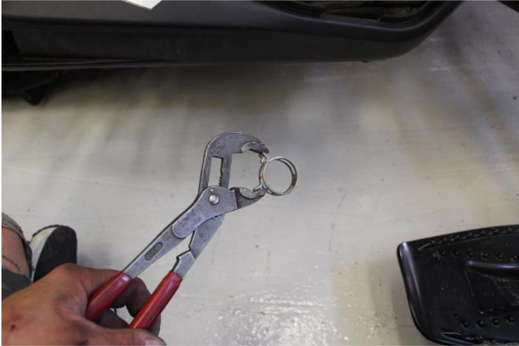
**Replace the stock clamp with a normal hose clamp supplied with the kit.**
