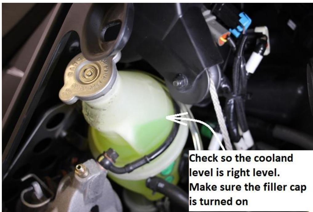
**Before you fill up antifreeze in the new radiator, check the coolant level. The filler cap must be closed when filling the radiator.**
