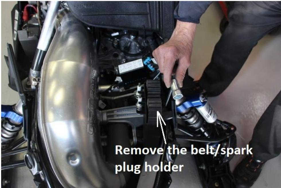
**To make space for the cooler kit you have to remove the holder for the spare spark plugs and the spare belt.**
