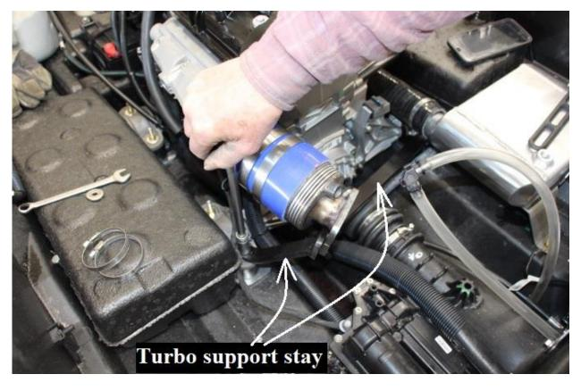
Tighten the nuts to the turbo support stay.
