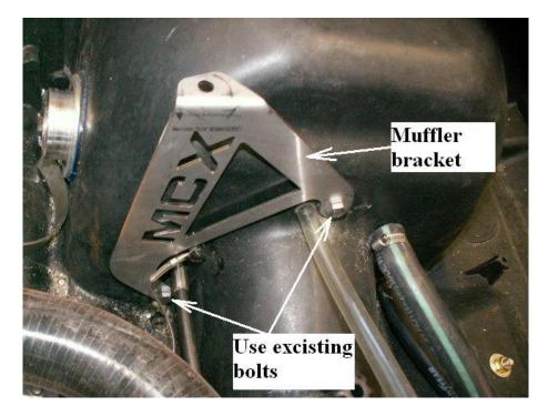
Install the muffler to the muffler bracket.
