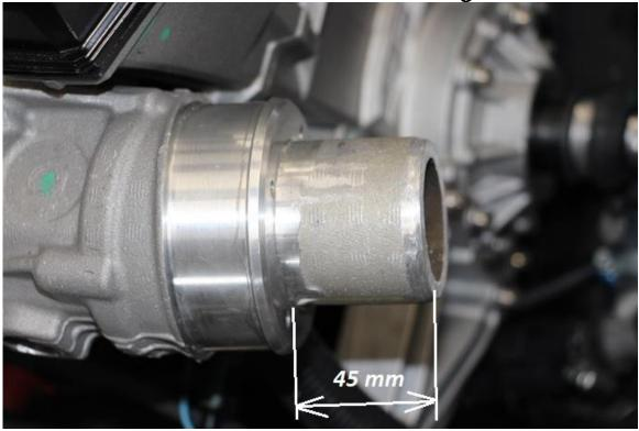
Before installing the exhaust headers, cut the end of the header so it remains 45 mm like the picture.
