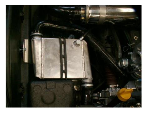
Install the intercooler to the intercooler bracket. Strap it down with the elastic rubber holder.
