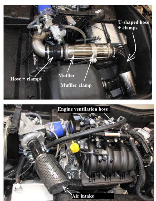
Install the air intake hose to the turbo inlet. Turn the hose so the engine ventilation nipple is facing forward/upper so it fits the new engine ventilation hose that you can install now. Use hose clamps to all joints. Install the air intake aluminium basket and the pre-charger air filter.Fill up the engine cooling system with anti freeze.
