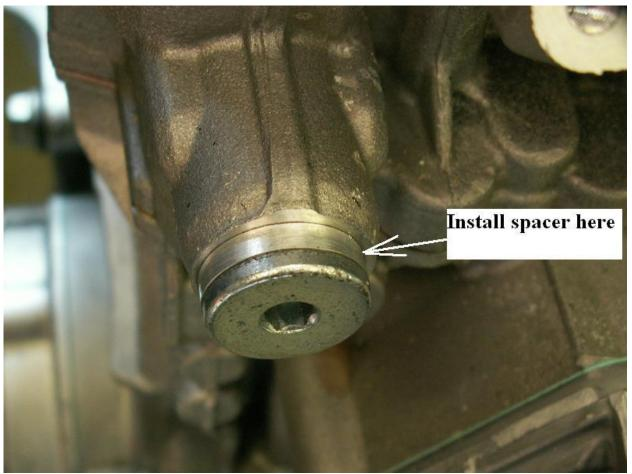
Install the cam chain tensioner.
