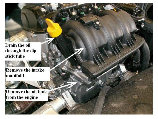
The reason why the oil tank must be removed is because a nipple for the oil return from the turbo shall be installed on the side of this tank.
