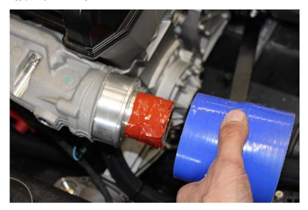
Put on the new hose to the exhaust manifold. And put on the original hose clamps.
