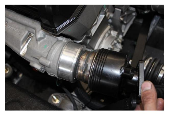
Try on the flexi pipe on the exhaust manifold and check so it fits. If it is to tight, adjust the end pipe of the alu-headers by grinding until it fits fine.
