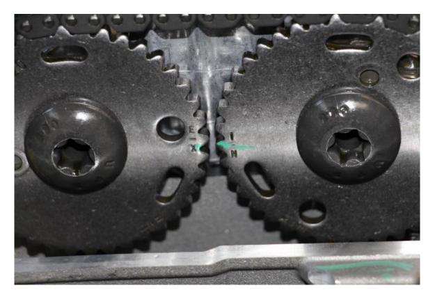
Rotate the crankshaft until piston number 2 is at top (=TDC) and the cams are positioned like the picture above.
