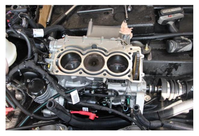
When the cylinder head is off, clean all the surfaces before you install the new, thicker head gasket.
