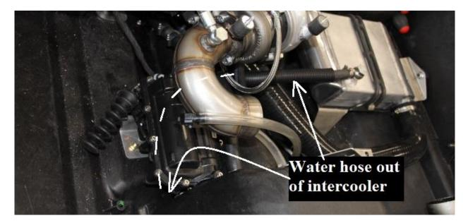
Demount the hose going out from the exhaust manifold and re-route it to the water outlet of the intercooler. Use banjo bolt + banjo fitting + 2 cupper washers supplied with the kit. Re-use the stock hose clamp.
