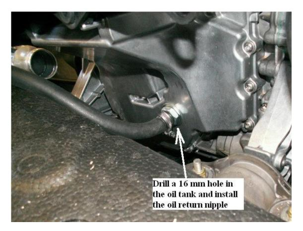
Install the 800 mm long oil return hose to the nipple. Secure with a hose clamp.
