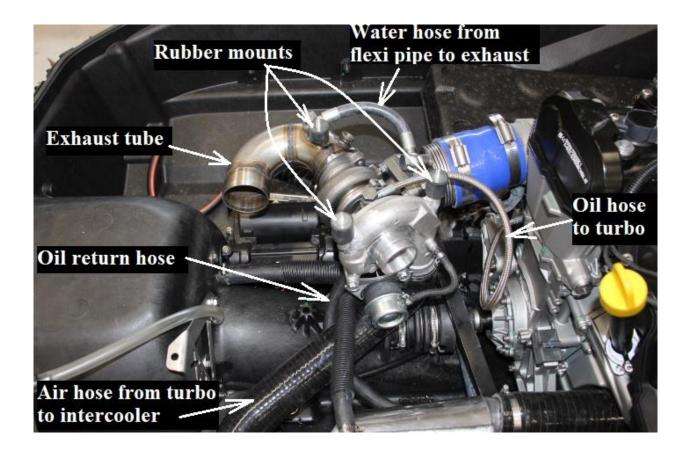
Install the exhaust tube going out from the turbo. (Don't forget the gasket) Install the water hose from the flexi pipe to the exhaust tube.
