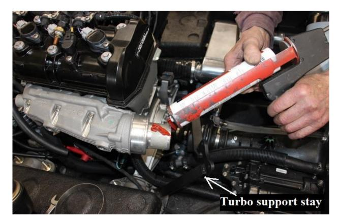
Apply the glue on the tip of the exhaust manifold.
