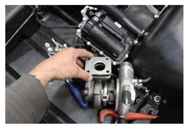
Now the turbo shall be installed. Check so the gasket is placed right before you install the turbo.
