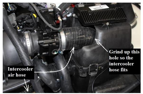
Install the U-shaped air hose going from the intercooler to the throttle body .The hole in the upper air box must be modified to make space for the air hose.
