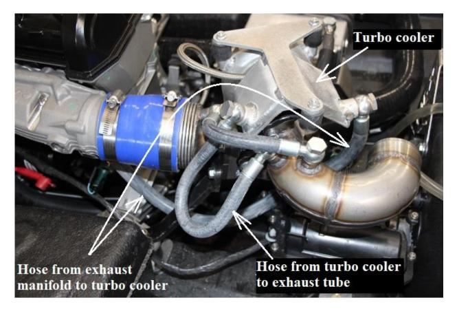
Install the turbo cooler on top of the turbo. Install the hoses going in and out of the cooler. (see picture)
