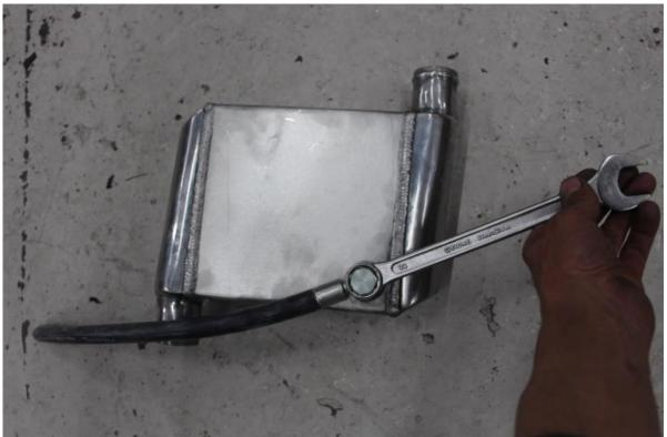
Before you put the intercooler in place, install the water on the lower side of the intercooler.
