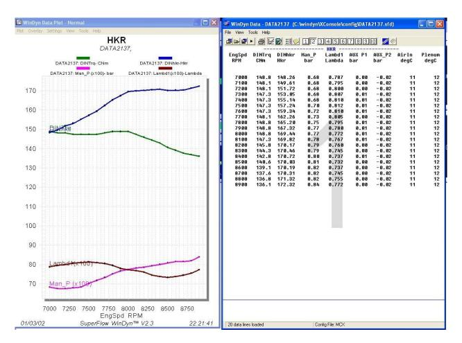
Using higher turbo pressure than 80 kPa may cause engine damages.
