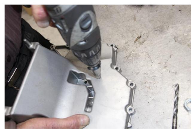
Find a plane surface for the nipple and drill a 16 mm hole. Install the oil return nipple + O-ring from the inside of the tank and tighten the nut from the outside. Use thread lock to secure the nut.
